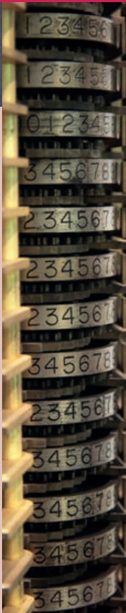
Detail of the calculating wheels, part of Charles Babbage's analytical engine.
